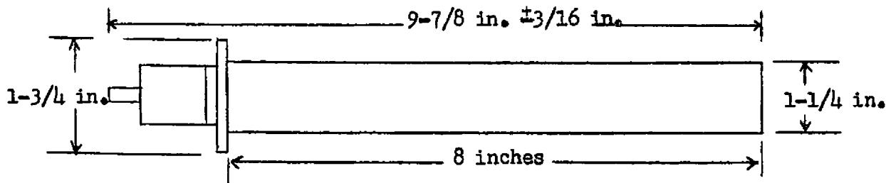
The 6353 is a corona regulator tube suitable for regulating very high voltages in moderate current power supplies.
