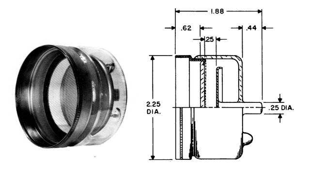
The FW-114 High-Current Phototube has a current output linear from 10<sup>-9</sup> ampere to 25 amperes
