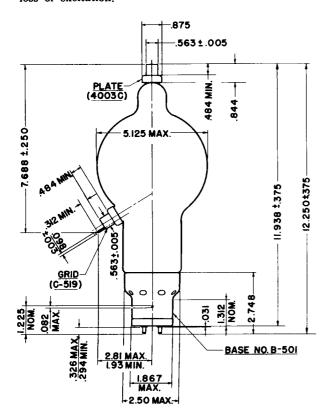
Grid Dissipation—The power dissipated by the grid of the 450TL must not exceed 65 watts. Grid dissipation may be calculated from the following expression:
