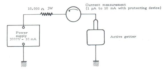
The active getter operation requires the use of a TV 19500 permanent magnet supplied with TV 19008 Focus Coil.
