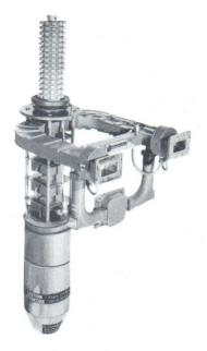
the collector being cooled by water vaporization according to the Vapotron technique \* which insures a high safety of operation.
