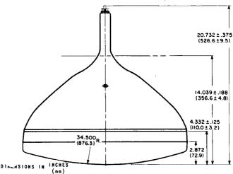
Note: In side view, spherical radius = 34,000 in (863.6 mm).
