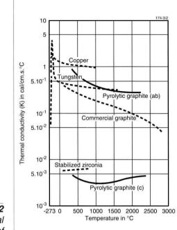
**Figure 2** Thermal conductivity of various materials
