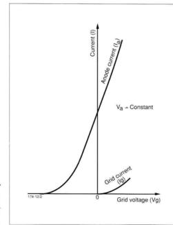
Figure 17 Grid influence on the anode current in a triode fact that small changes in the grid voltage can cause large excursions of the anode current has led to this basic grid being called the control grid.
