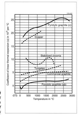
*Figure 3* Thermal expansion coefficient of various materials
