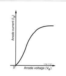
Figure 16 Characteristics of a diode zone. In fact, the presence of electrons near the cathode modifies the electric field produced by the anode. The current varies according to the Langmuir law :
