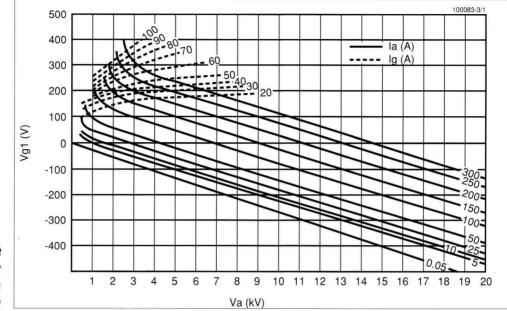
Figure 18 Constant-current characteristics of a triode
