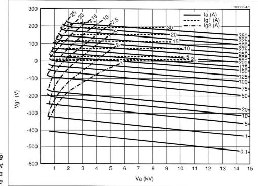
Figure 19 Constant current characteristics of a tetrode
