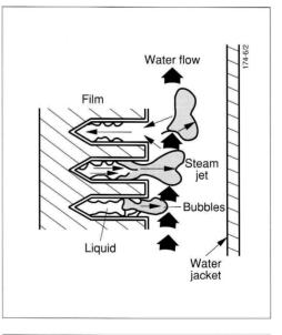
Figure 7 Hypervapotron anode cross section, showing operation
