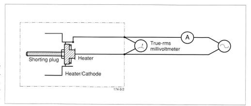
Figure 15 Correct setup for measuring the heating circuit resistance These are to assist in the appropriate heater transformer design, and assume no other cathode heating factors interfere.
