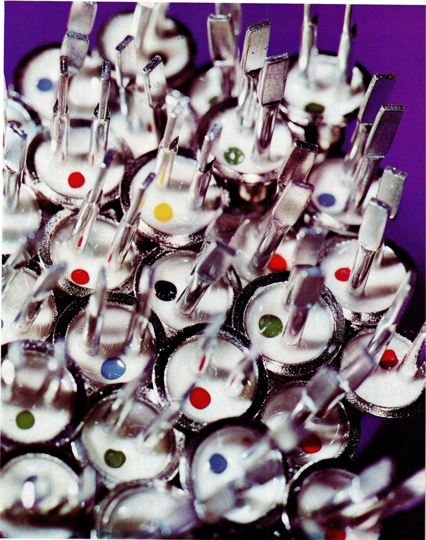
Fig. 4 The 10 tolerance groups are indicated by different colored dots as shown in Table 1
