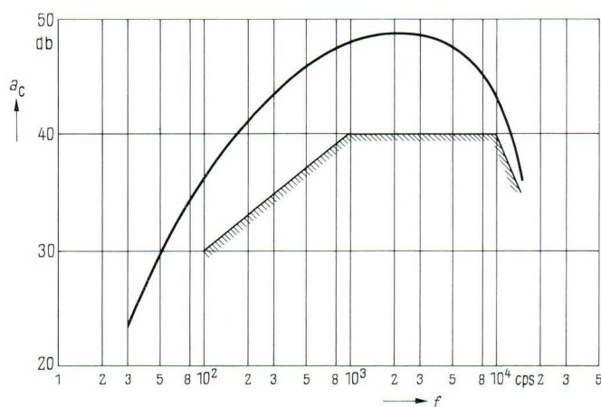
Fig. 3 Crosstalk attenuation a_c of the stereo decoder for transistorized broadcast receivers as a function of frequency
