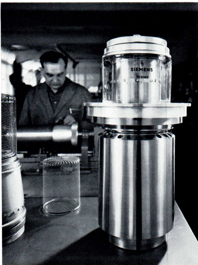
Fig. 1 High-power transmitter triode RS 2041 with mesh grid and ready-to-assemble cathode and grid construction
