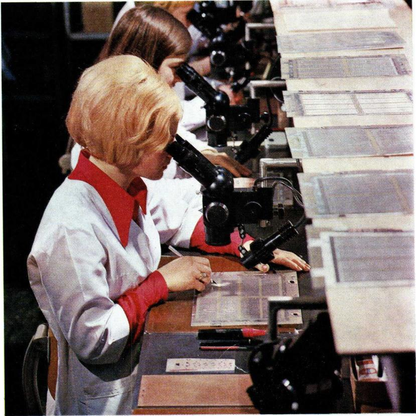
*Inspection of conductor pattern.*
