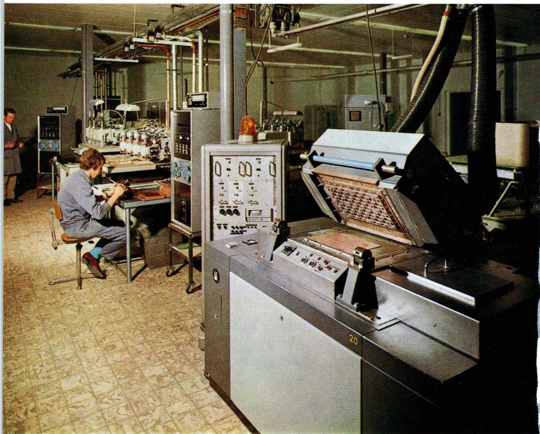
*Forty-spindle automatic jig drilling machine (foreground).*
