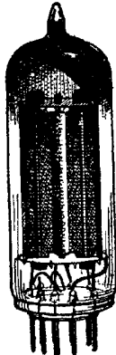
Rectifier valve or tube, giving full-wave rectification.
