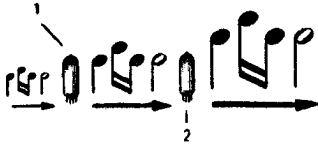
1 = 1st tube. 2 = 2nd tube. By means of these two tubes a double amplification will take place.
