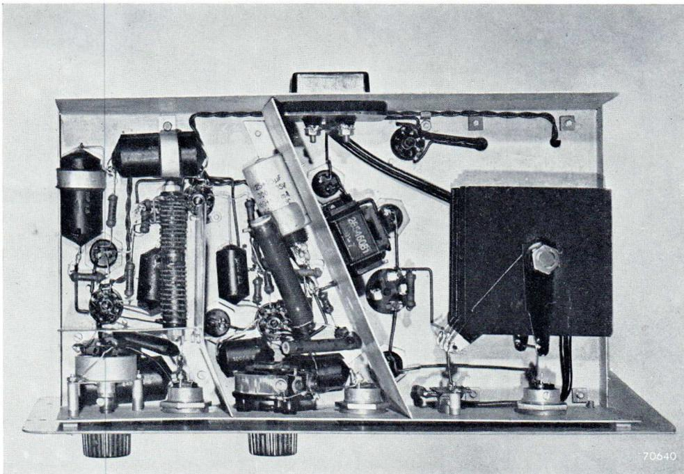
Fig. 62. Under-chassis view of the phototube amplifier.
