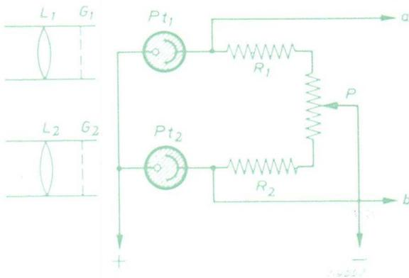
Fig. 53. Schematic diagram of and „Aniseikon”.  $L_1$  and  $L_2$  form the binoculars with the gratings  $G_1$  and  $G_2$  behind. The scene is projected on the cathodes of the phototubes,  $Pt_1$  and  $Pt_2$ , the photo current is balanced with the potentiometer  $P$ . When something in the scene alters, the balance is upset and a voltage difference occurs between  $a$  and  $b$ .
