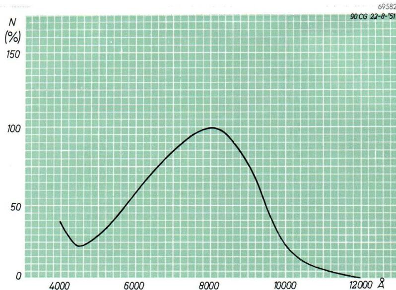
for incandescent light with a colour temperature of 2700 °K, 20  $\mu$ A/lm, but for daylight, which usually has a much smaller infra-red component the sensitivity is only 4  $\mu$ A/lm. The daylight sensitivity of a phototube with an "A" type cathode, however, is about 80  $\mu$ A/lm, whilst for a lamp with a colour temperature of 2700 °K it is 45  $\mu$ A/lm.
