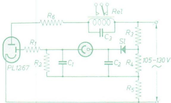
Fig. 43. Circuit diagram of relay amplifier with trigger tube PL 1267.
