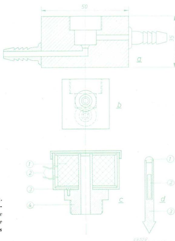
Fig. 52. Cross sectional drawings of the solenoid valve. a and b — the plexi-glass holder; c the screw cap where in 1 — the winding; 2 — the connection leads; 3 — the iron housing; 4 — the screw nut; d — the plug; 1 — the top plug; 2 — the loose iron core and 3 — the plexi-glass plug.
