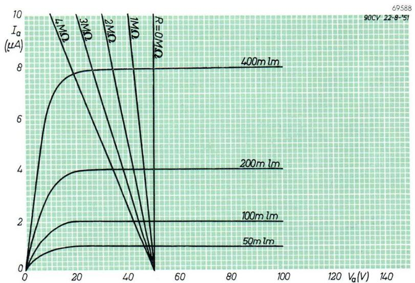
Fig. 15.  $I_a/V_a$  characteristic.
