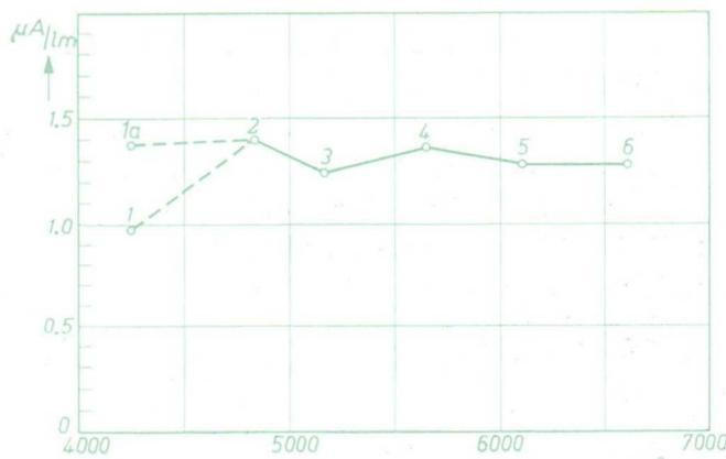
Fig. 74. Overall sensitivity of the spectro-photometer described.
