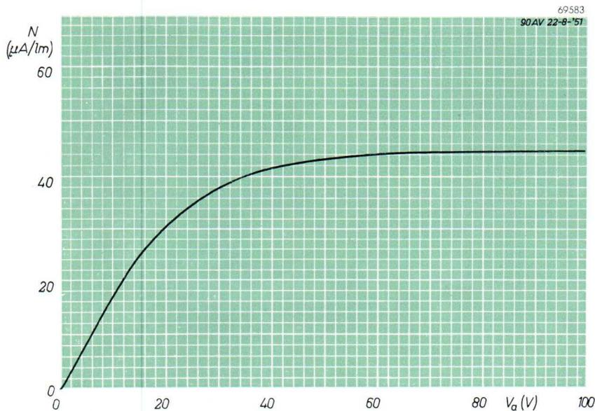
Fig. 3. Saturation characteristic of a high-vacuum phototube.
