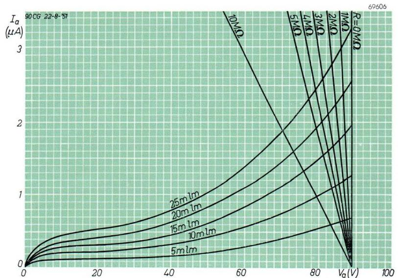
Fig. 30.  $I_a/V_a$  characteristic.
