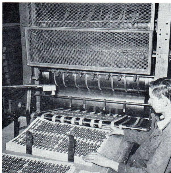
*Close up of the scanning head of the photo-electric counter. Underneath the belt part of the light-projector can be seen.*
