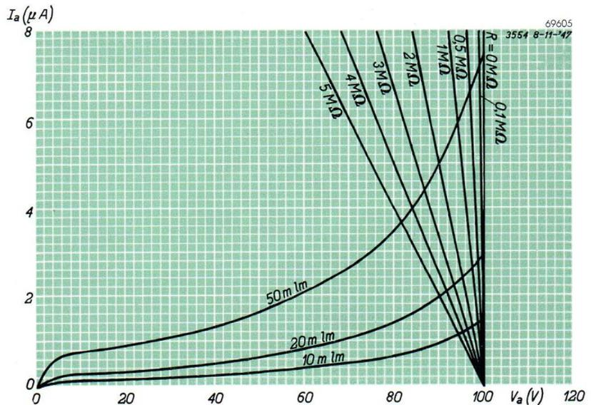
Fig. 36.  $I_a/V_a$  characteristic.
