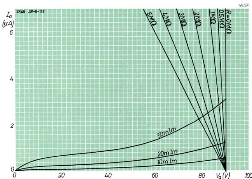
Fig. 20.  $I_a/V_a$  characteristic of gas-filled phototube.
