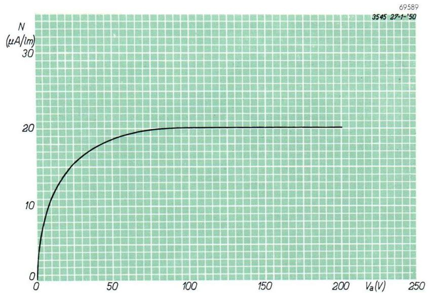
Fig. 18. Saturation characteristic.
