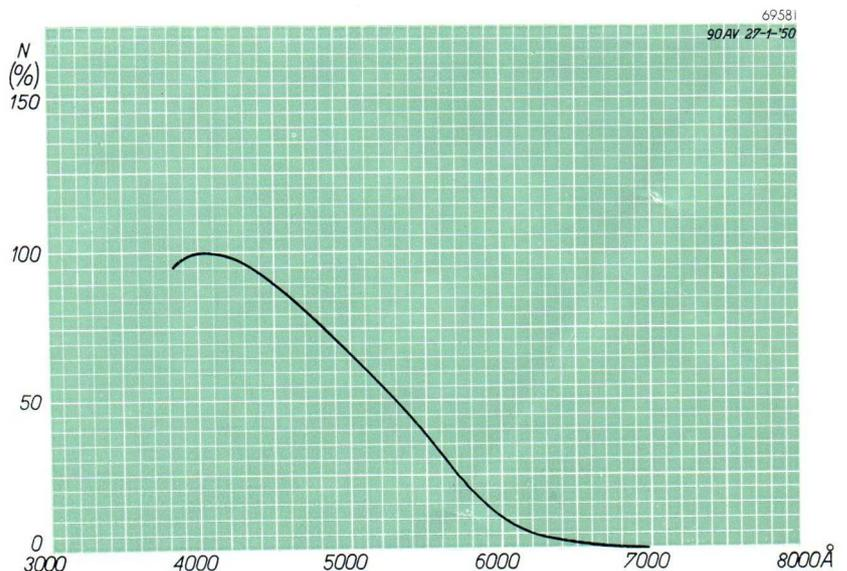
Fig. 2. Spectral response curve of phototube with "C" type of cathode.
