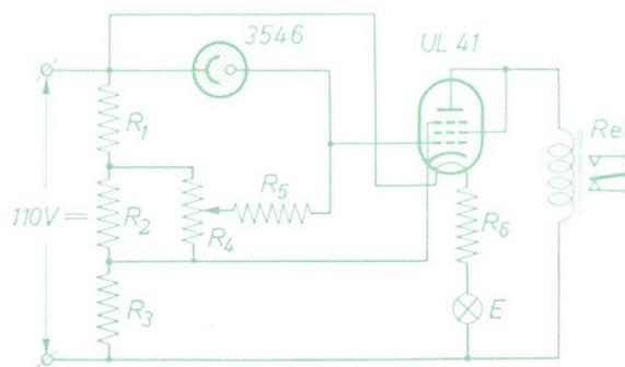
Fig. 42. Circuit diagram of 110 V D.C. relay amplifier with tube UL 41.
