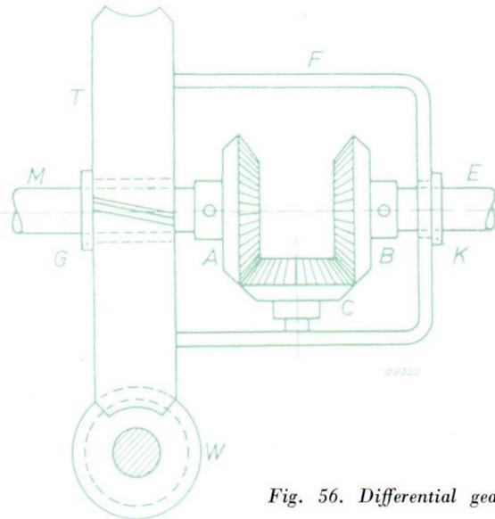
Fig. 56. Differential gear.
