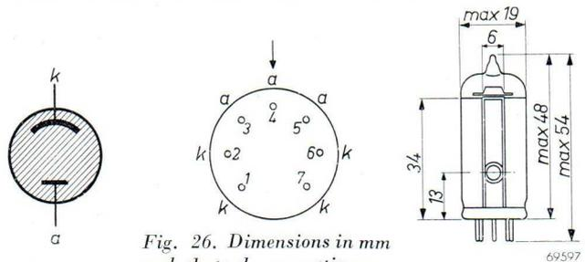
Fig. 26. Dimensions in mm and electrode connections.
