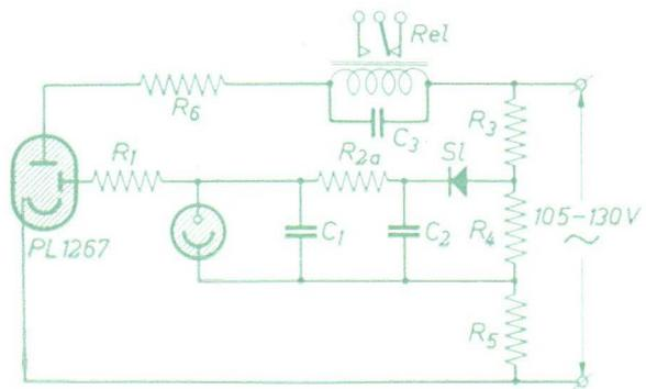
Fig. 44. Circuit diagram of relay amplifier with trigger tube PL 1267.
