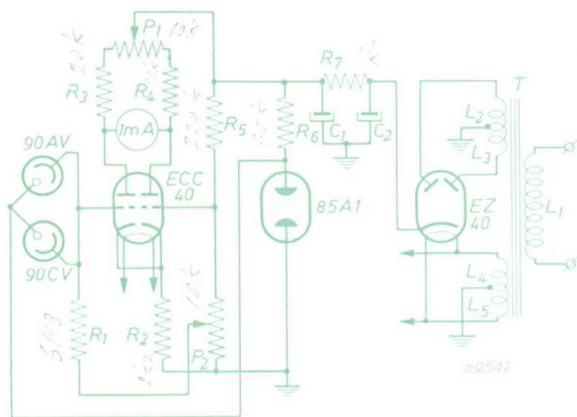
Fig. 76. Circuit of the V.T. voltmeter to be used with the spectro photometer.
