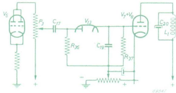
Fig. 67. Diagram of one half of the bridge circuit.
