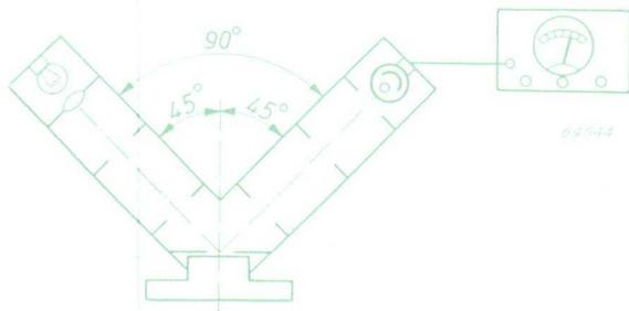
Fig. 72. Photometer for comparative measurement of washings.
