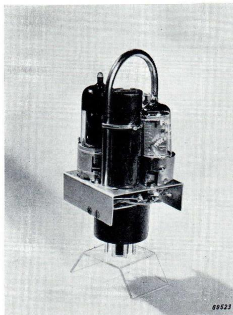
Fig. 39. Compact relay amplifier with tubes EF 40 and PL 21 mounted on an octal base.
