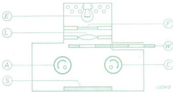
Fig. 75. Arrangement of a simple spectro-photometer, for comparative colour measurements.
