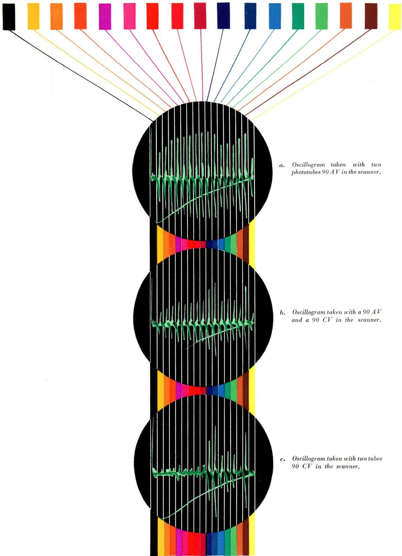
a. Oscillogram taken with two phototubes 90 AV in the scanner.
