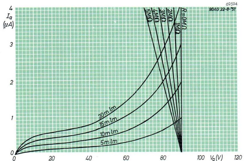
Fig. 27.  $I_a/V_a$  characteristic.
