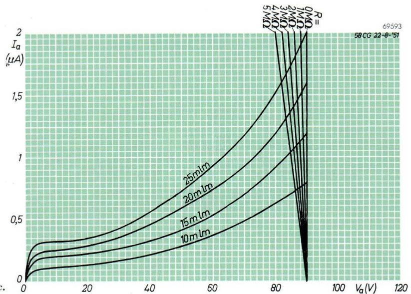
Fig. 24.  $I_a/V_a$  characteristic.
