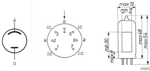
Fig. 13. Dimensions in mm and electrode connections.
