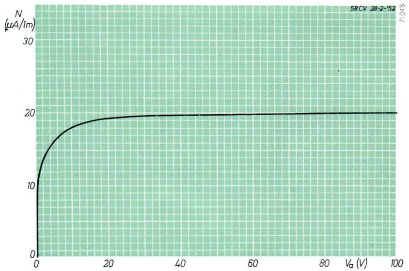
Fig. 6. Saturation characteristic.
