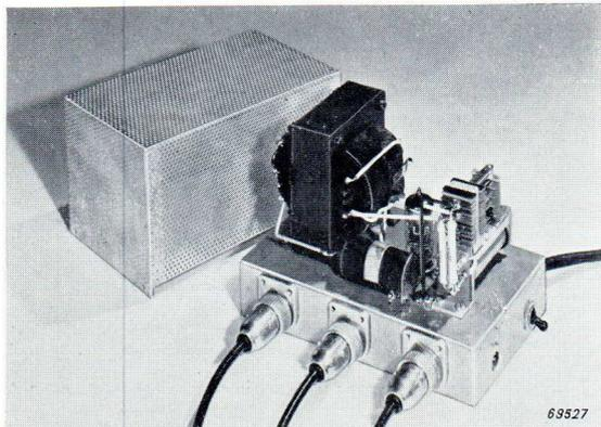
Fig. 48. Phototube amplifier for smoke detector with perforated hood removed.
