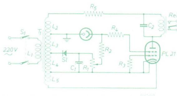
Fig. 41. Circuit diagram of an electronic switch with thyatron PL 21.
