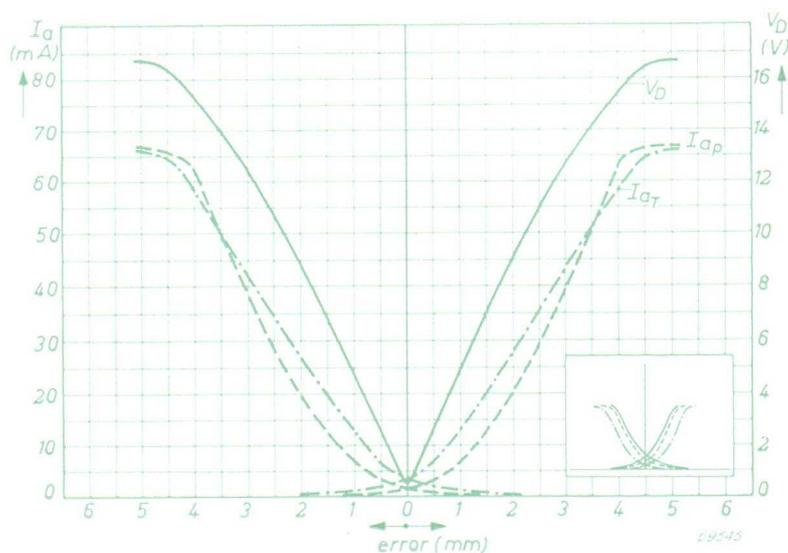
Fig. 69. Voltage on the diodes ( $V_D$ ) and the anode current ( $I_a$ ) of the power stage, as a function of the error. The curves marked  $I_{ap}$  are for pentode connection, those marked  $I_{at}$  for triode connection of the power tubes.
