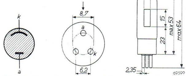
Fig. 32. Dimensions in mm and electrode connections.
