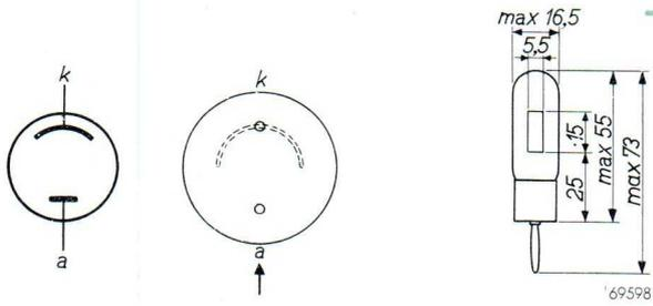
Fig. 17. Dimensions in mm and electrode connections.
