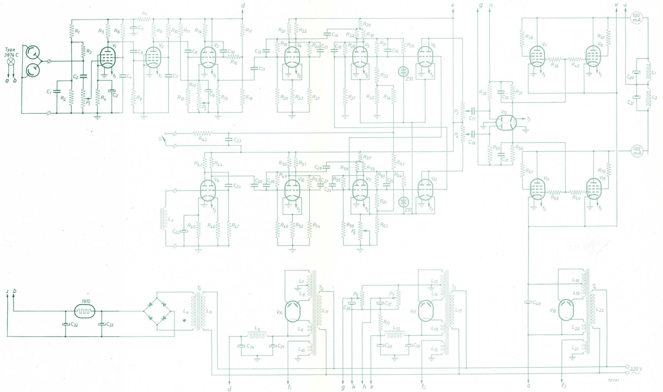
Fig. 70. Circuit diagram of the electronic register control apparatus.
