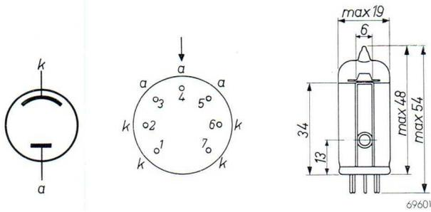
Fig. 9. Dimensions in mm and electrode connections.
