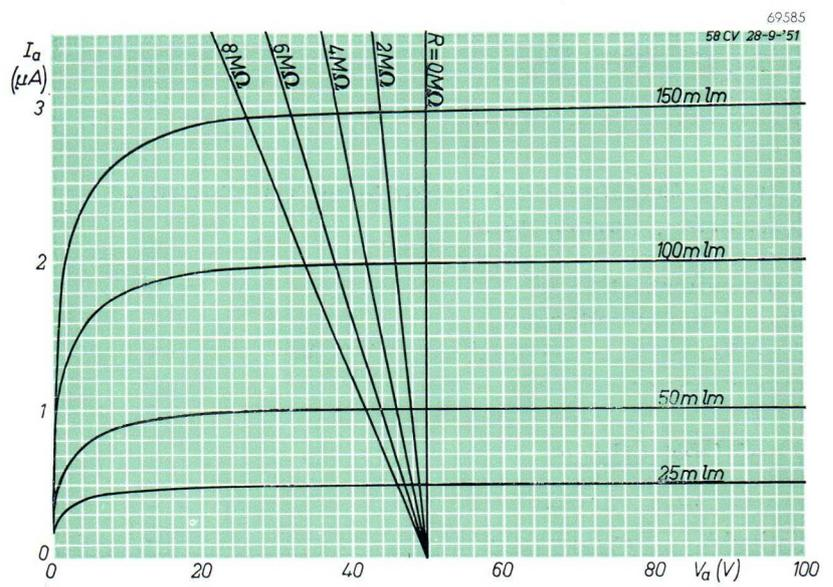
Fig. 7.  $I_a/V_a$  characteristic.
