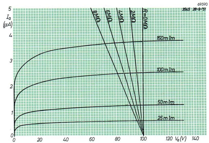
Fig. 19.  $I_a/V_a$  characteristic.
