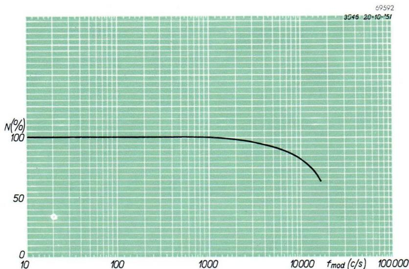
Fig. 21. Frequency characteristic of gas-filled phototube.
