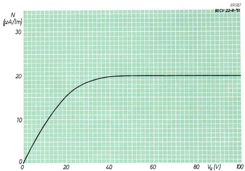
Fig. 14. Saturation characteristic.
