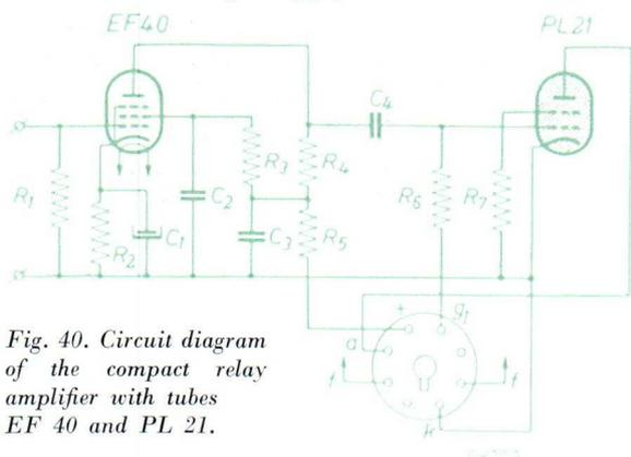
Fig. 40. Circuit diagram of the compact relay amplifier with tubes EF 40 and PL 21.
