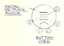
PIN 2 GRID No.1 PIN 10 GRID No.2 PIN11-CATHODE PIN12-HEATER HD.PLATE - ANODE
