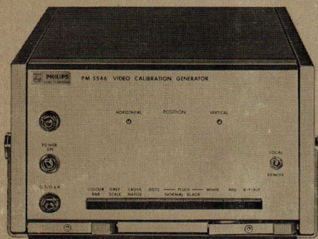
PM 5546 video calibration generator which provides high-precision test signals for TV studio and transmitter work
